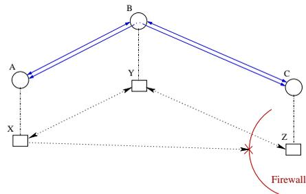
**Fig. 3.** Overcome asymmetric connectivity by using the name-to-path discovery service. Since node A cannot connect directly to node C, it looks for a path through node B. On the left hand side we show pseudo-code representing the steps at node A.
