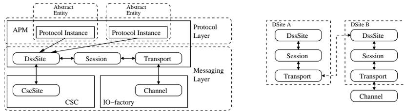
**Fig. 2.** To the left, the layout of the DSS and its three separate software subcomponents. The protocol layer and parts of the messaging layer are located in the same software subcomponent, the APM. The figure also depicts the location of the sub-objects that represent the DSite structure. The APM does abstract messaging and the CSC/IO-factory does the actual messaging. The figure to the right, depicts how a DSite A uses DSite B to construct a virtual circuit.
