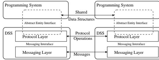
**Fig. 1.** The structure of the DSS middleware library. The figure depicts two processes sharing data structures using the DSS. The distribution model for the two programming systems is on the level of shared data structures. Within the DSS, the protocol layer exchanges protocol operations with other protocol instances. The bottom layer of the DSS, the messaging layer is responsible for passing the protocol operations to the correct process.
