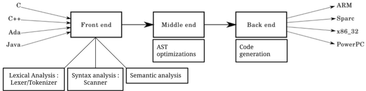
Figure 3.1.: Schematic representation of a classic compiler model<sup>1</sup>
