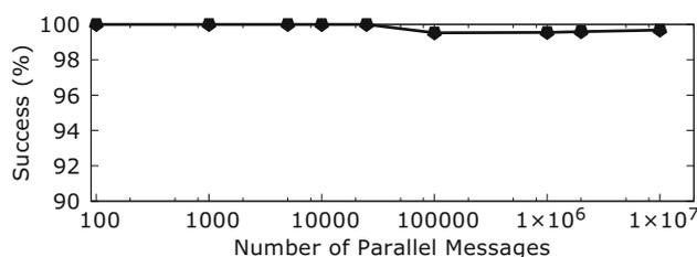
**Fig. 10** Success rate of an *SD-CPS* controller vs. number of messages processed in parallel
