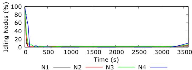
**Fig. 9** Idling nodes during a parallel execution of 1 million workflows
