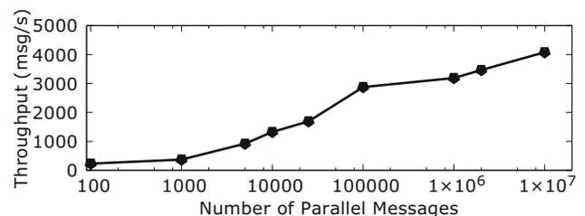
**Fig. 11** Throughput of an *SD-CPS* controller versus number of messages processed in parallel
