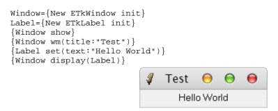
Figure 3-12. A sample ETk application using object orientation.
