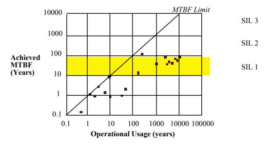
COTS software data from nuclear, chemical and aerospace (control and protection) industries. Claimed MTBF is limited to the total usage time. Some systems exhibit growth rates 100 times less than the best case.
