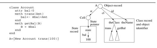
Figure 13: An object with one attribute and two methods
