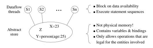
Figure 6: Computation model of OPM
