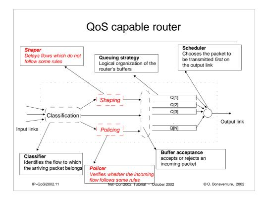
In practice, the shaper could also be located on the output link, but we don't address this issue here to keep the picture simple and understandable.
