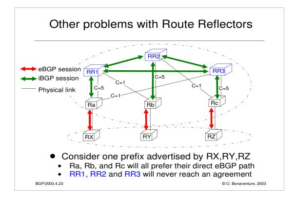
With an iBGP full mesh, all BGP routers would received the three possible paths and RR1 would prefer the path via R2, RR2 would prefer the path via R3 and RR3 would prefer the path via R1.
