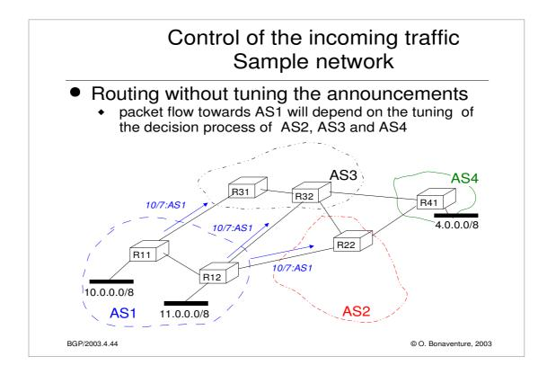
In this example, we assume that no filters are applied by AS2, AS3 and AS4 on the routes received from AS1.
