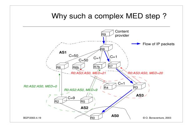
•In the example above, assuming a full iBGP mesh inside AS1 and that all routes have the same local-pref value, router R8 will receive four paths to reach router R0 :
