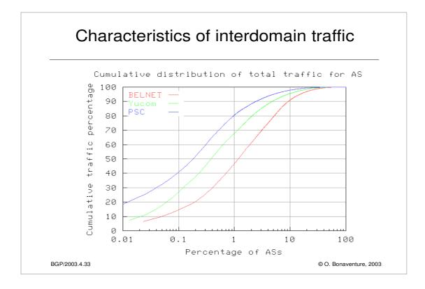
This figure is based on a study of all the interdomain traffic of three distinct ISPs at different periods of time. The trace was collected during one week for BELNET, the Belgian Research ISP, five days for YUCOM, a dialup ISP based in Belgium and one day for PSC, a gigapop in the US. This figure is analyzed in :
