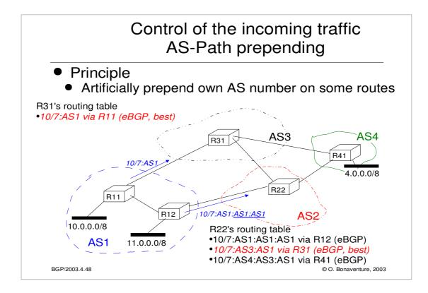
AS-Path prepending is a popular technique since in the BGP decision process, the selection of the shortest AS-Path is one of the most important criteria. In theory, the length of the AS-Path is not necessarily an indication of the quality of a path, but some studies have shown that, on average, short AS-Paths offered a better performance that longer paths.
