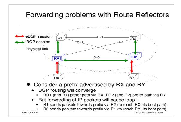
Note that this forwarding problem does not occur if R1 and R2 use some tunneling mechanism (e.g. MPLS) to send packets towards RX and RY via RR1 and RR2
